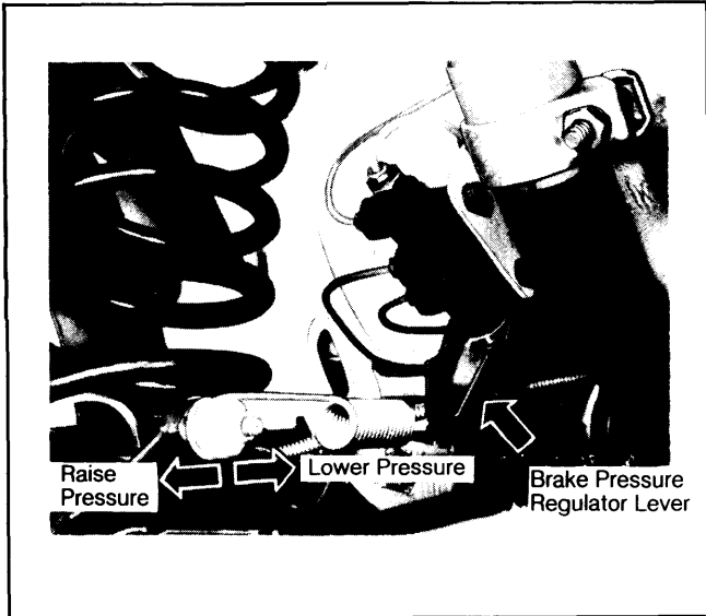
Fig. 3: Brake Pressure Regulator Adjustment
