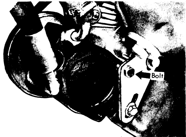
Fig. 6 Installed View of Power Steering Pump
